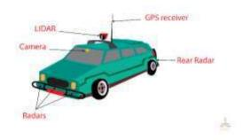
2) **Cameras** are to the front, sides and the back of the car for a complete 360 degree visual.
